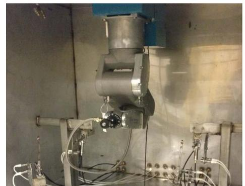
Robot arm with high pressure nozzle for precision detail cleaning
