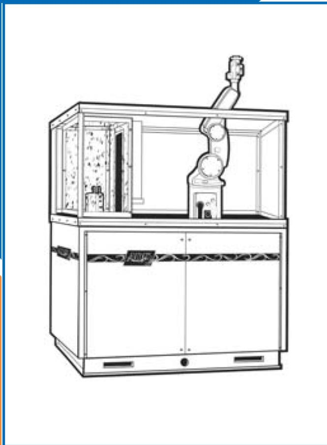
The next generation of parts washers is the integration of robots into cleaning operations. This may include a pick and place robot placing parts on a conveyor, a robot-operated spray nozzle cleaning a fixed part, or a robot manipulating a part over a fixed nozzle. Any combination of washing, rinsing, and drying can be combined into a cleaning cycle. Opening a door to place a part inside a cabinet is one example.
