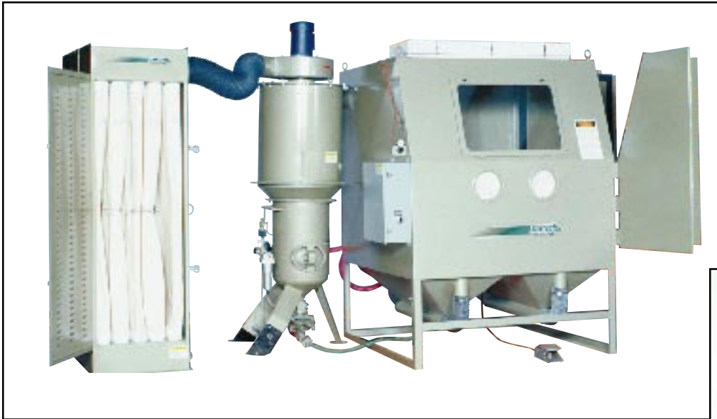
Model BNP-720 with 900 CFM Reclaimer and Dry Filter Dust Collector
